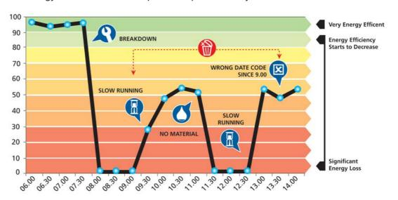
Implementing an OEE system provides the monitoring and indicators to enhance the overall efficiency of a factory in terms of productivity, quality and energy consumption.
